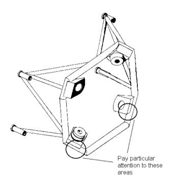
2. Perform a magnetic-particle inspection of the engine mount for cracks. Repair or replace any engine mount found cracked before further flight.
