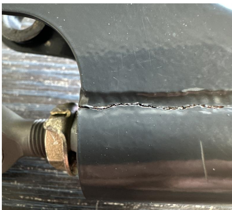
Figure 1 Cracked Pilot Cyclic Base P/N G41-42-801
