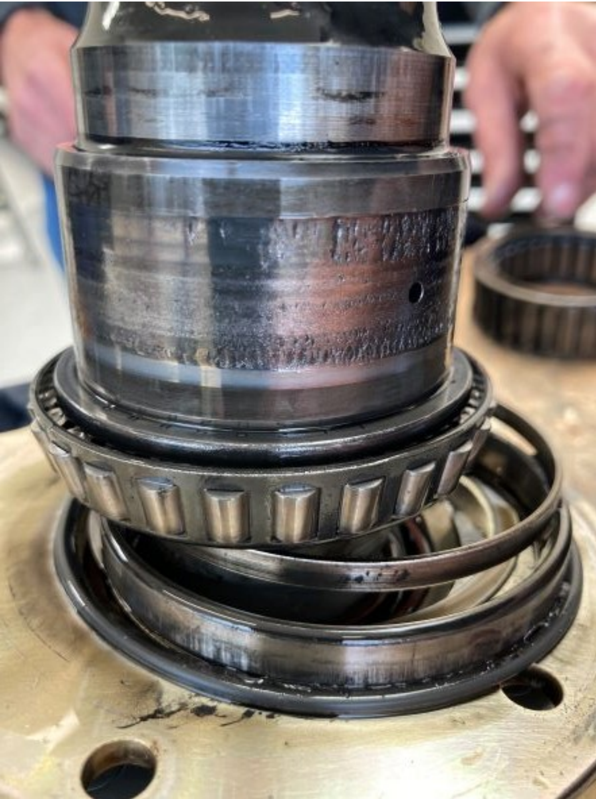
Shaft P/N C166-5 - Spalling damage.
