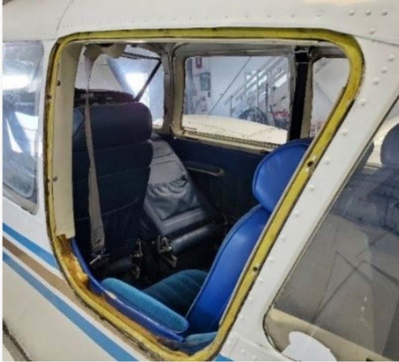
Picture 2 – Emergency exit window removed (Source: TSB A19Q0091)
