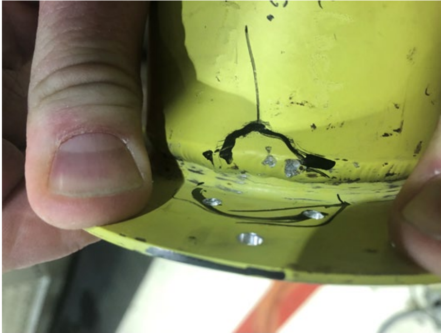
Figure 1: Cracked area of flange radius shown in circled area
