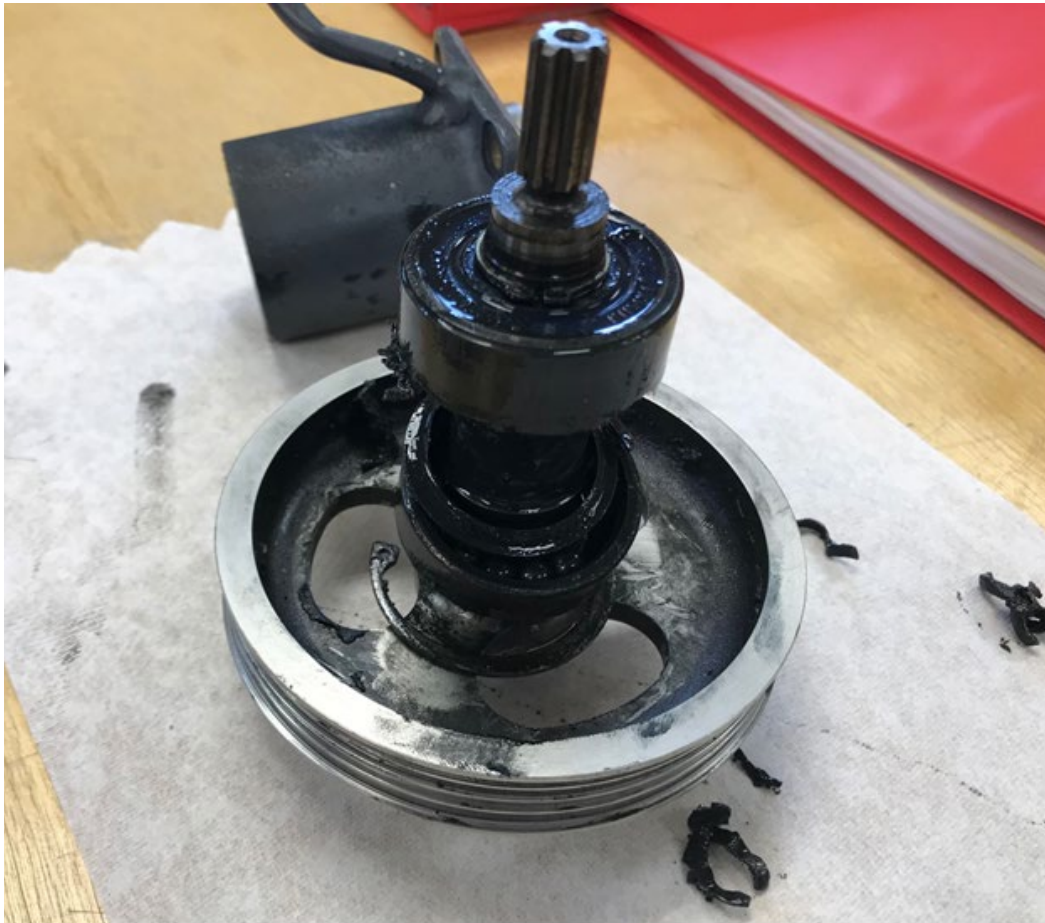
Picture 1 – Alternator pulley drive shaft, bearing failure
