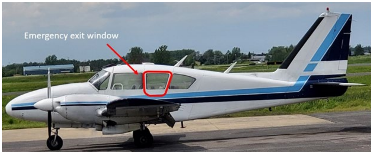
Picture 1 – Side view of the Piper PA-23-250 aircraft showing the emergency exit window (Source: TSB A19Q0091)
