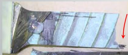
(b) Failure surface –OML side
