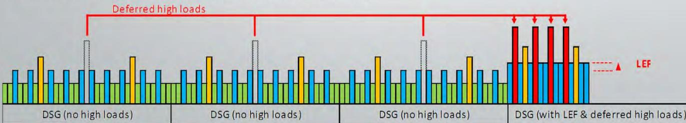
Cycles below composites truncation level (green) are eliminated after 3 DSG
