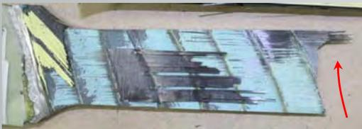
(c) Failure surface –IML side
