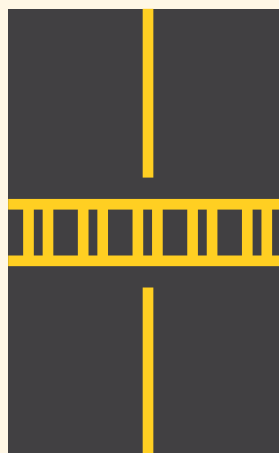
// Runway holding position marking – Pattern B
