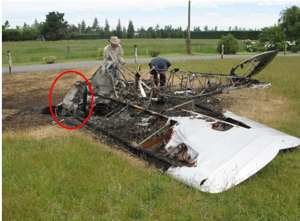
Figure 2: Position of the ruptured fuel tank.
