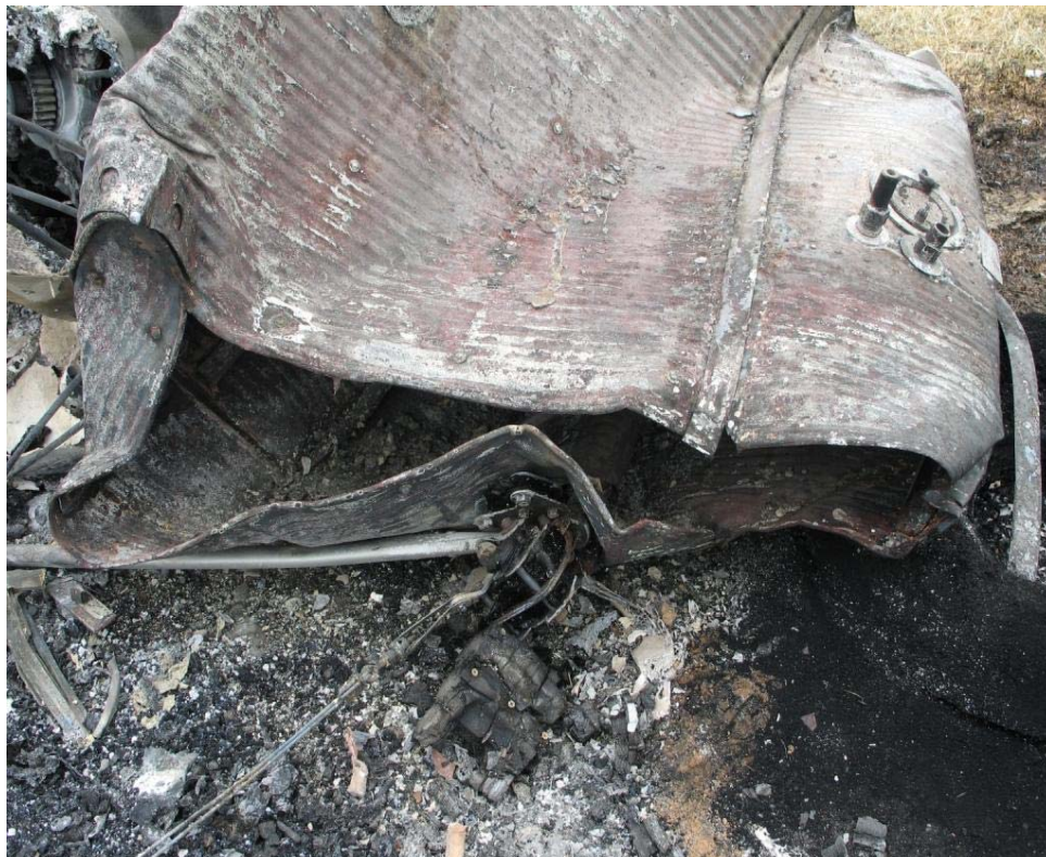
Figure 1: Open side seam (right side) of fuel tank.
