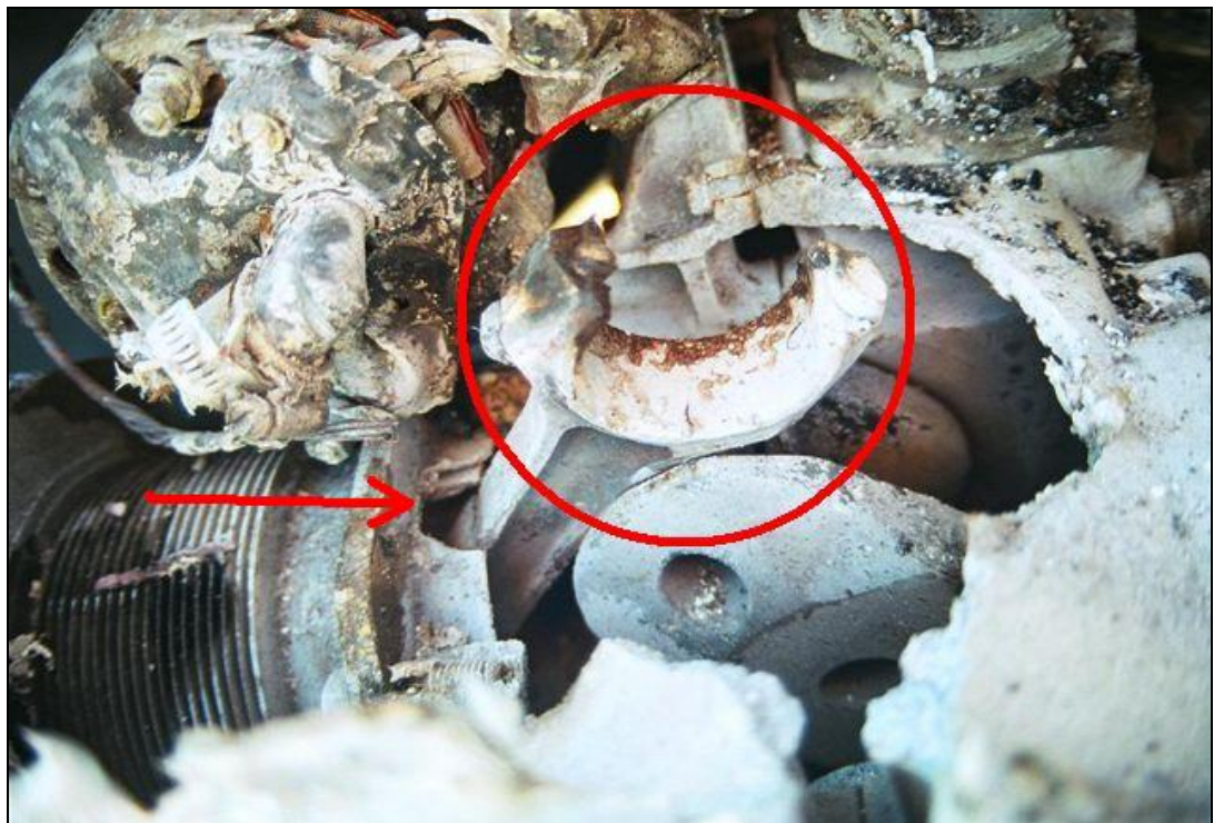
Fig 2: Failed con-rod big end bearing (circled). Arrowed area shows damage resulting from continued engine running in this failed condition.
