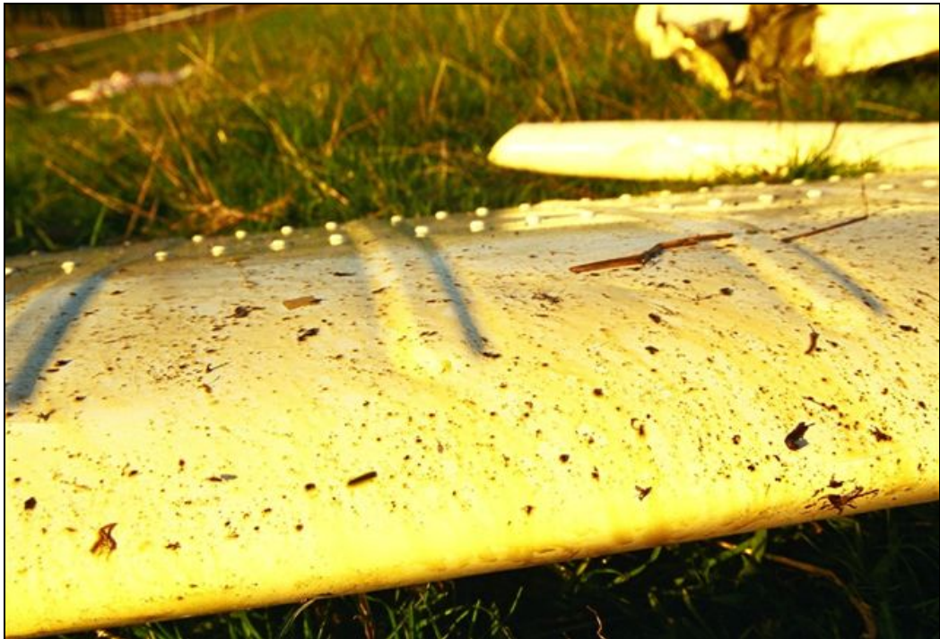
Fig 4 Considerable amounts of engine oil covered the tail boom and stabilizer.
