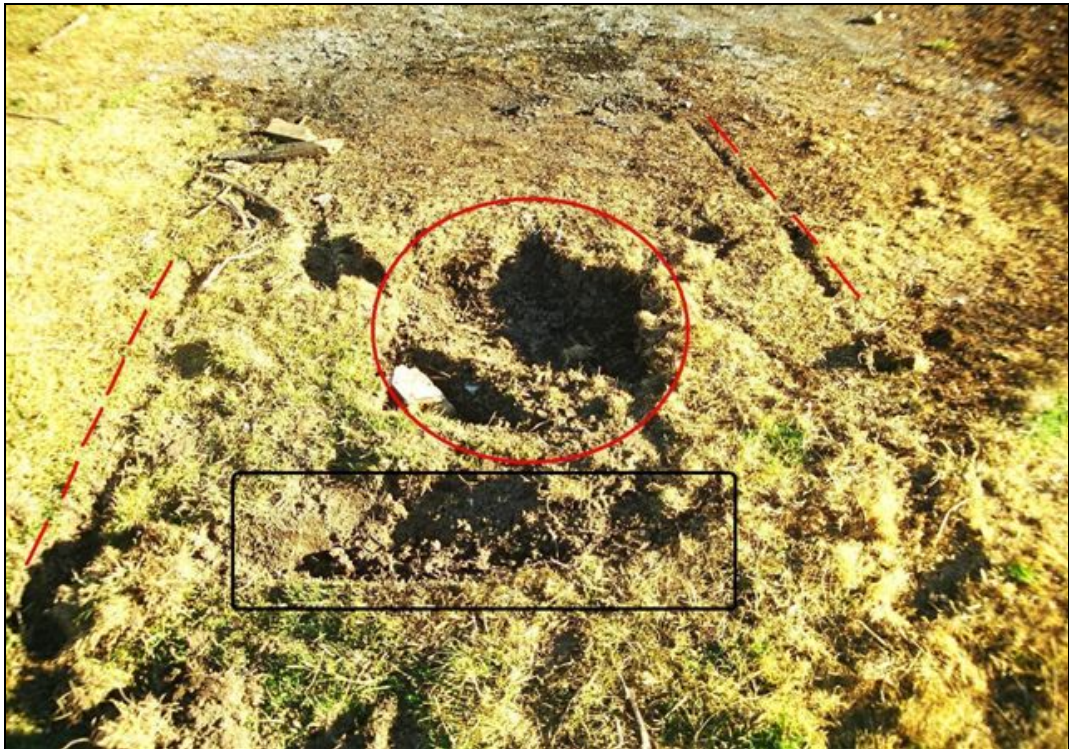
Fig 3: Severity of Impact: Black rectangle outlines rear cross tube ground scar, and red circle indicates engine contact. Both landing gear skids impressions are clearly visible next to red dashed lines.
