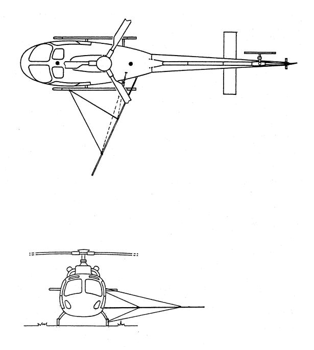
Diagram 1: Spray equipment configuration as approved (Only one side shown for clarity)
