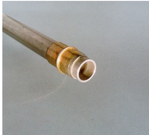
Figure A4 Properly formed tube end (new) (Permissible deformation is visible inside tube end)
