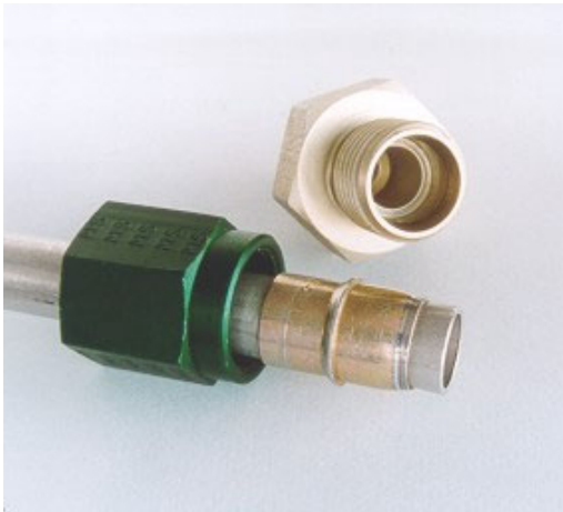
Figure A3 MS flareless fitting components (Tube, MS21921 nut, MS21922 sleeve, MS21916D reducer)
