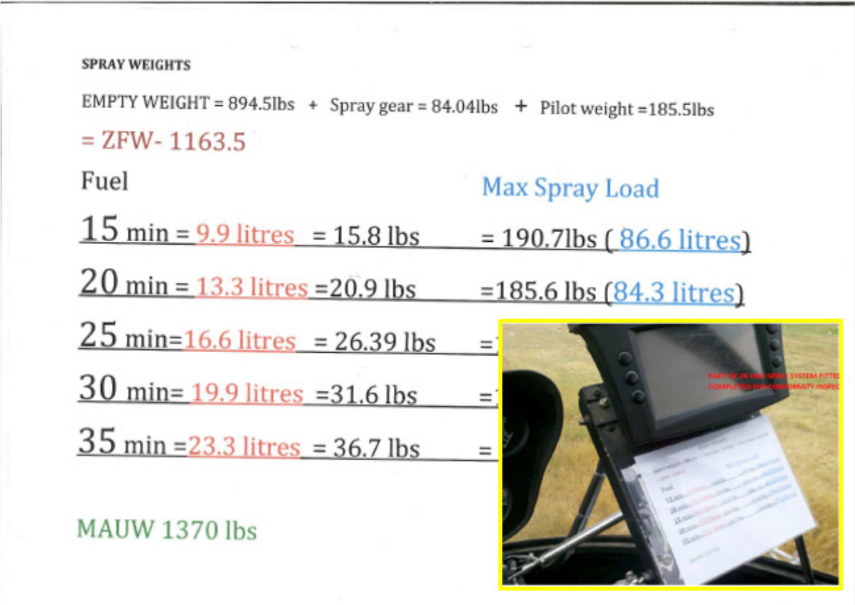
Figure 2. Spray Weights quick reference card found at scene (Inset: card pictured in ZK-HWJ).
