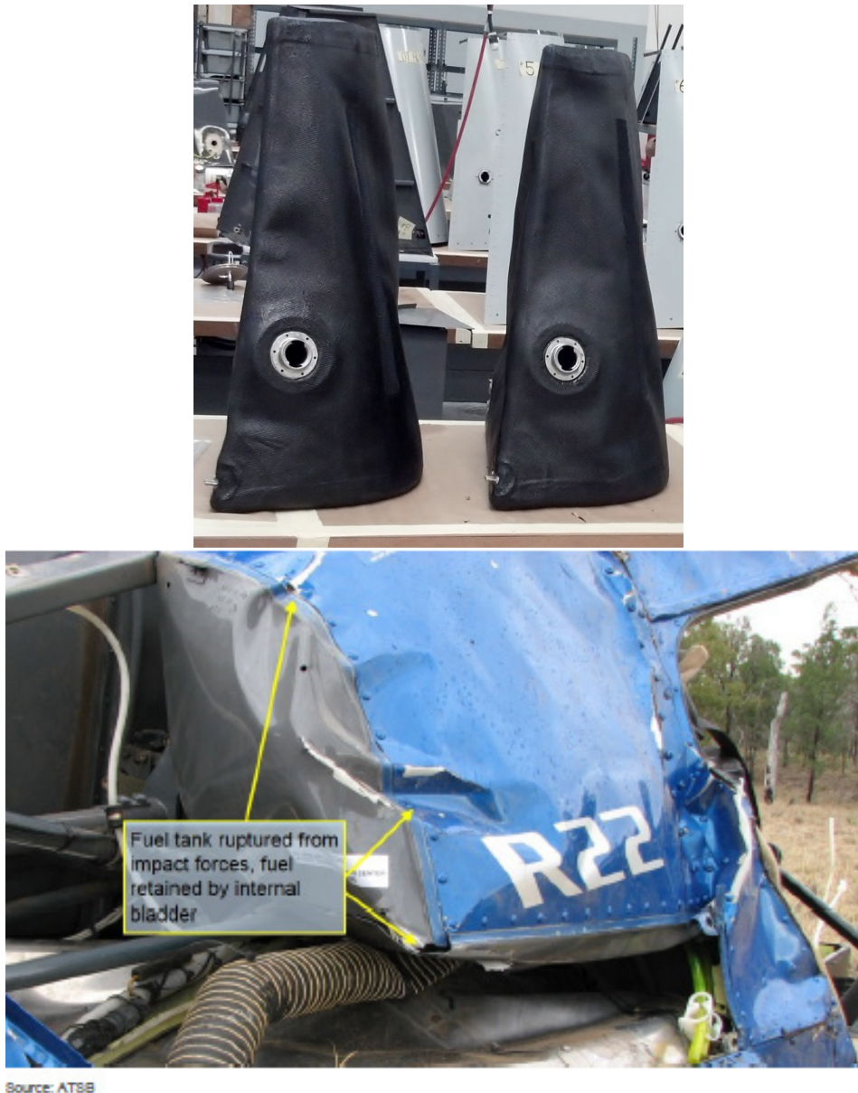
Figure 4. Bladder fuel tanks for compliance with SB-109 and post-impact evidence.
