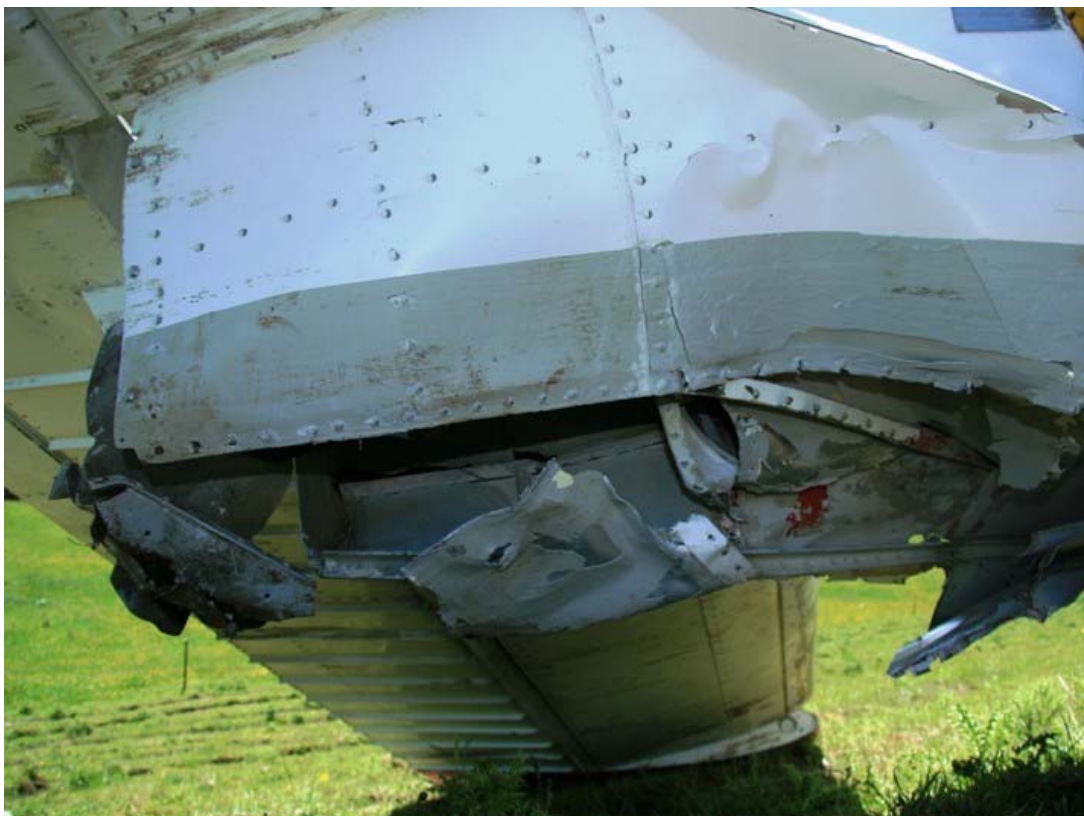
Figure 2: Damage to aft fuselage caused by fence strike
