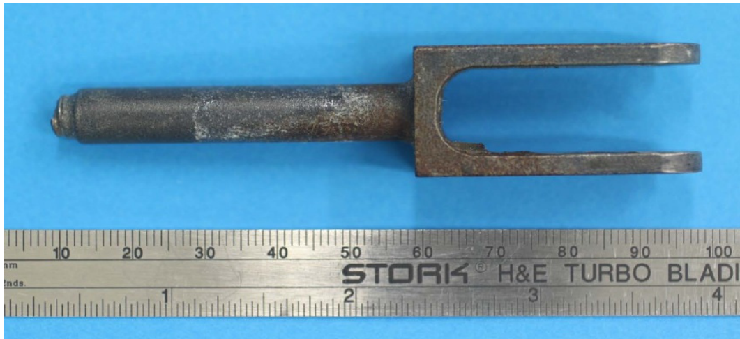
Figure 2: Failed upper end fitting
