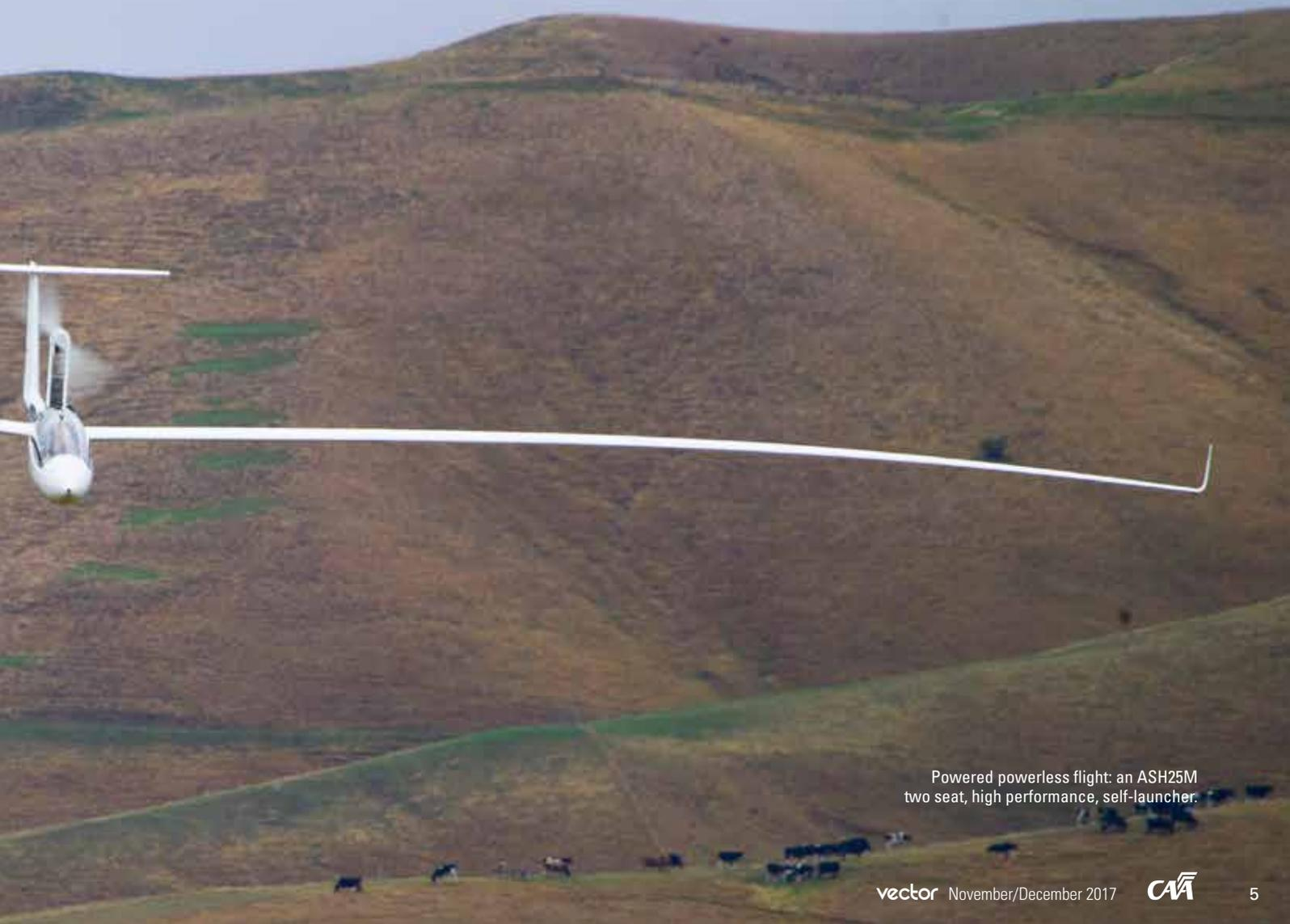
Powered powerless flight: an ASH25M two seat, high performance, self-launcher.
