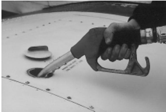
The fuel pump nozzle should be kept in contact with the side of the filler neck at all times while fuel is being delivered. This ensures that a potential difference does not develop between the area surrounding the filler neck and the nozzle.
