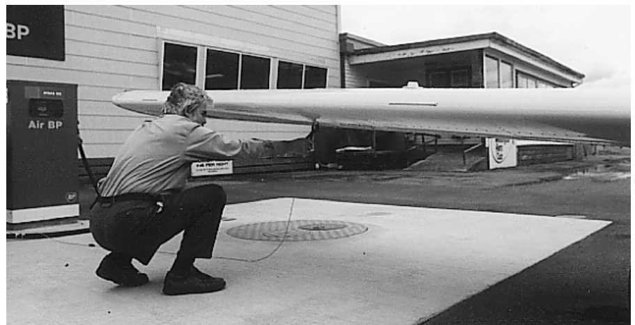
Securely attaching the bonding wire to a non-painted metallic surface (one that can convey an electrical charge to or from the aircraft fuel tank) before refuelling begins will equalise any potential difference that exists between the aircraft and the fuel pump.
