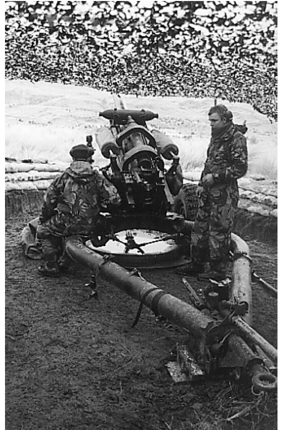
A long barrel L-118 Light Gun in action in the Waiouru Training Area (NZM301). This gun is capable of firing a projectile a distance of up to 18 kilometres.
