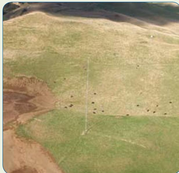
From the photograph, it can be seen that this mast is very hard to see even in good weather. The ground at the site is approximately 300 feet **amsl** (100 metres), and the mast height is just under 200 feet **agl** (60 metres). If the pilot had been at 500 feet **amsl** over the sea, then the turn inland would indeed have been a hazardous manoeuvre. Now there's a lesson.
