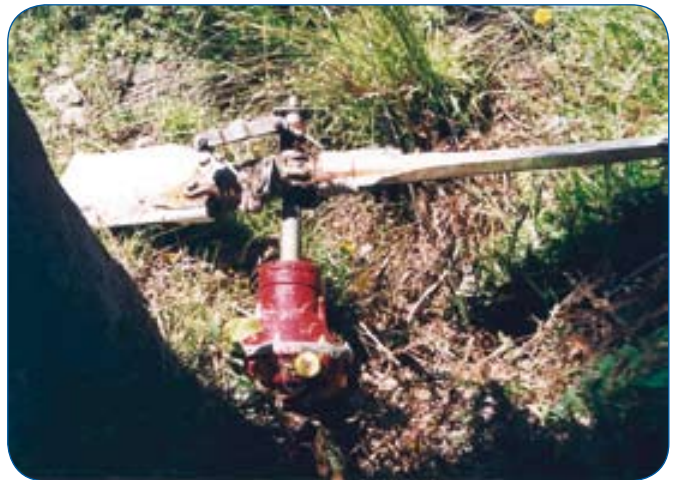
The result of the strike was the departure of the tail rotor and 90-degree gearbox from the airframe.
