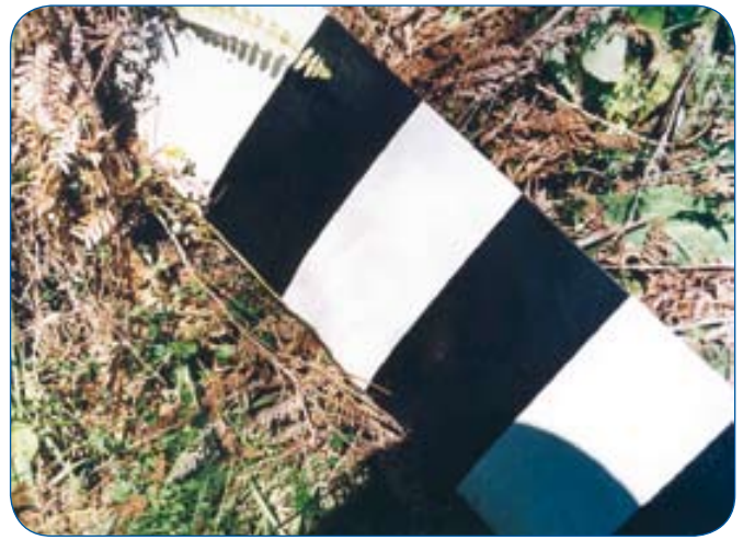
The seemingly minor dent on this Iroquois tail rotor blade was caused by a flailing longline that had been picked up by the main rotor.
