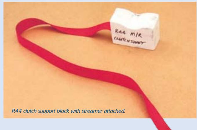
R44 clutch support block with streamer attached.
