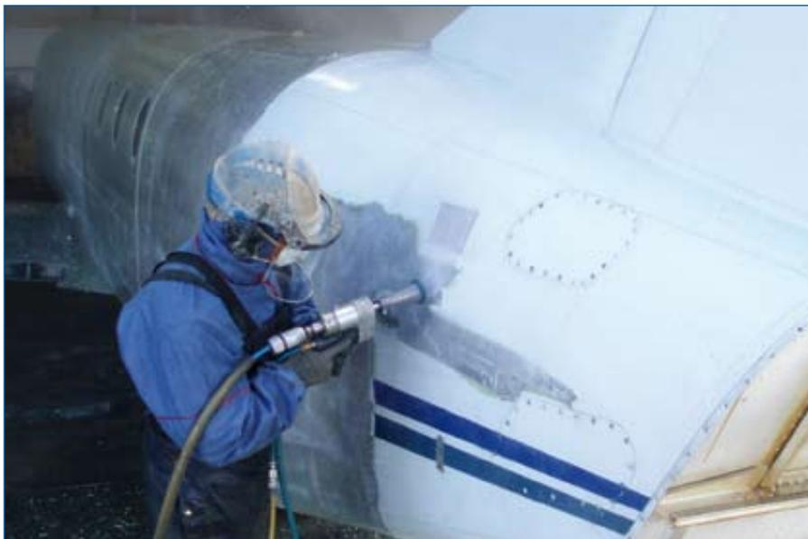
Hydroblasting uses ultra-high pressure water to remove paint.
