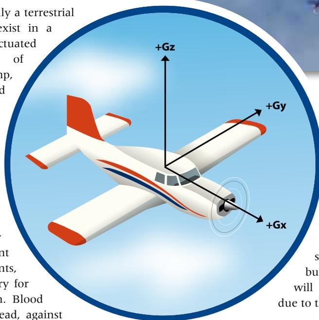
aircraft. For example, the CT-4 is limited to operating between +5.5 Gz and -1.8 Gz, while the Cessna 152 'Aerobat' is rated from +6.0 to -3.0 Gz.
