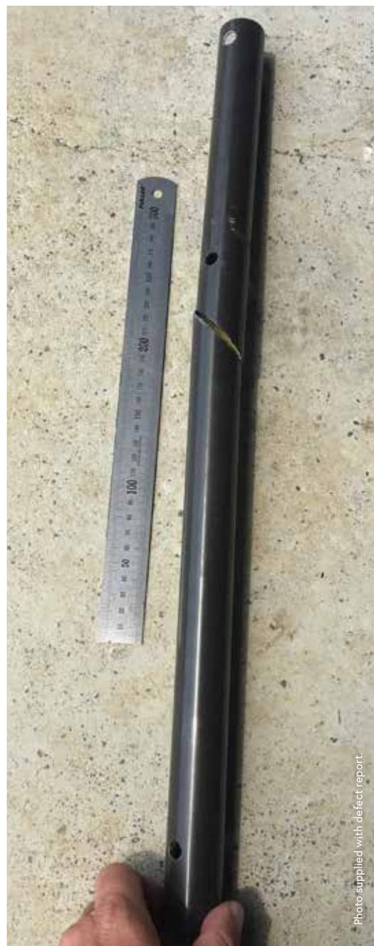
// Continuing airworthiness notice 27-014 was issued in February 2020 to "bring attention to a defect reported to the CAA of finding a severely cracked pilot to co-pilot tail rotor torque tube on a Hughes 369FF".
