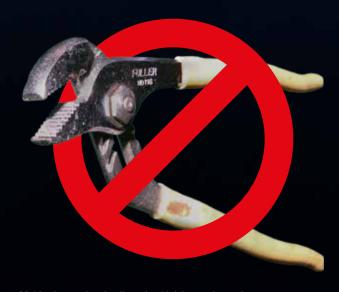
Multi-grip or poly grip pliers shouldn't be used anywhere on any aircraft. They can damage the fitting too easily.
