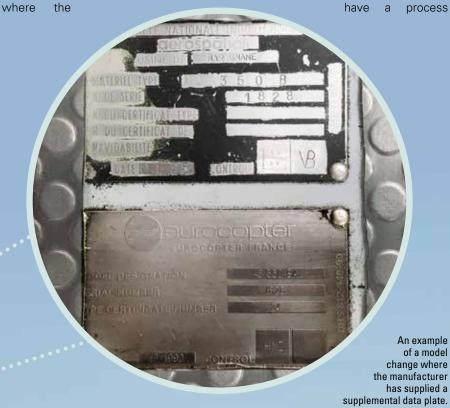
manufacturer authorizes the replacement of a fuselage as a spare part with its own part number and possibly a component data plate.
