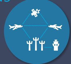
he CAA is proposing that ADS-B OUT be mandatory in controlled airspace for aircraft above FL 245 by the end of 2018, and by the end of 2021 for aircraft below FL 245.
