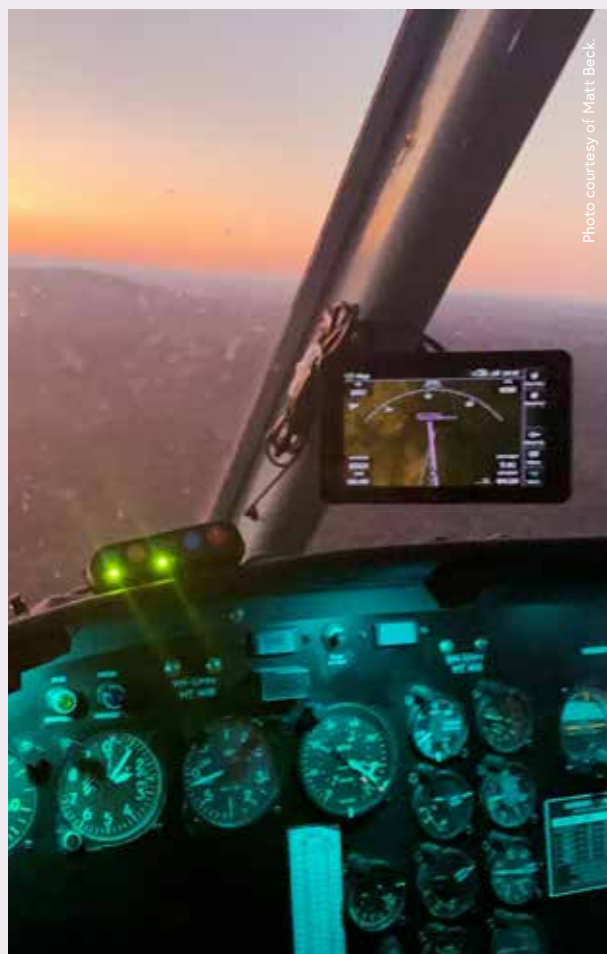
// A permanently mounted GPS – an example of a design change.
