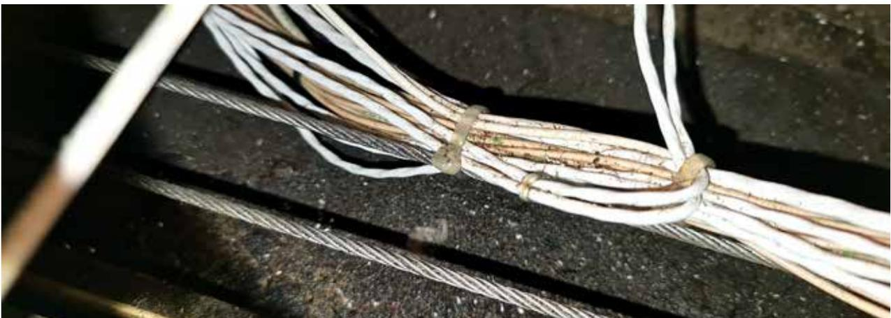
// Wiring bundle attached to a flight control cable – note the metal shavings on the wire.
