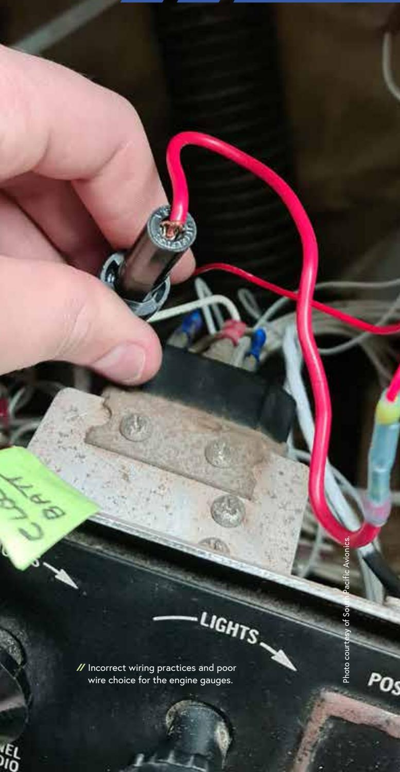
// Incorrect wiring practices and poor wire choice for the engine gauges.
