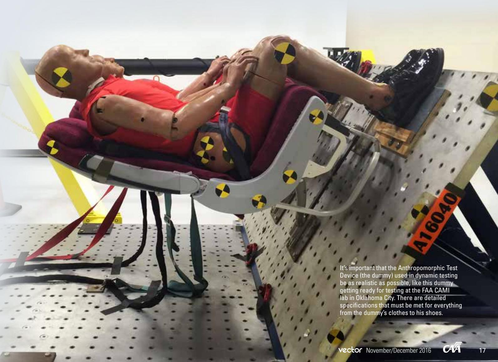
It's important that the Anthropomorphic Test Device (the dummy) used in dynamic testing be as realistic as possible, like this dummy getting ready for testing at the FAA CAMI lab in Oklahoma City. There are detailed specifications that must be met for everything from the dummy's clothes to his shoes.
