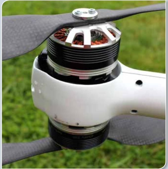
The coaxial propulsion arrangement on the SkyJibX4.
