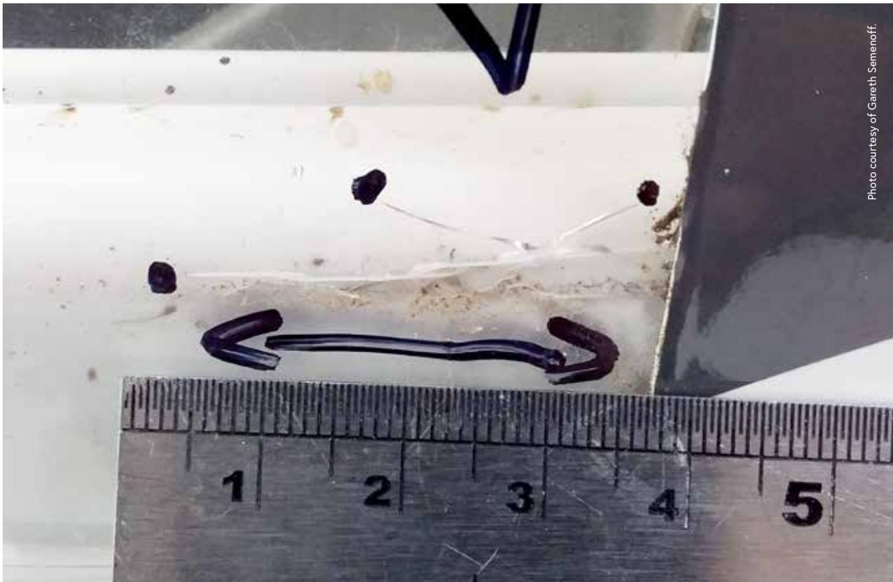
// A Taranaki engineer found this cracking in the Aeroprakt windscreen he was about to replace. The CAA was able to warn the rest of the Aeroprakt community with a continuing airworthiness notice, after the engineer reported it as a defect.
