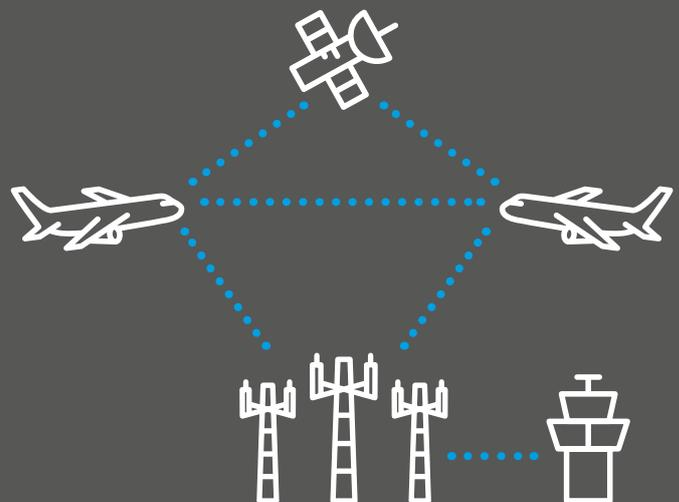
An on-board transponder broadcasts an aircraft's position, altitude, and velocity directly to air traffic control. Richer and more accurate information than that from current transponder systems means more efficient traffic management and improved safety.
