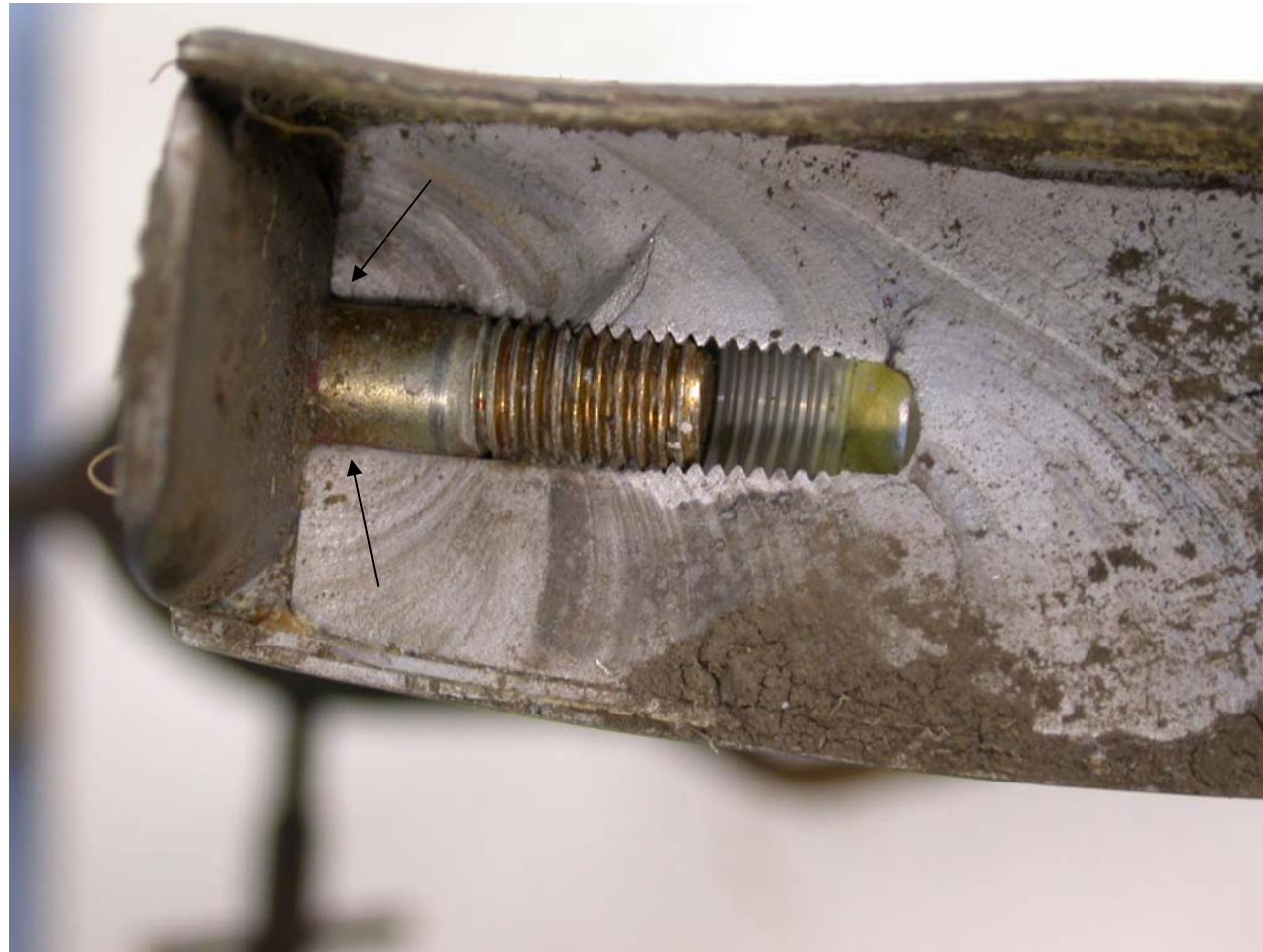
Figure 6. The fracture through the root fitting. The arrows indicate the location of the fracture origins on both sides of the bolt hole very close to the leading edge.
